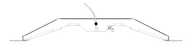
Return the wiring cover to the closed position and use the twist locks to secure the cover
