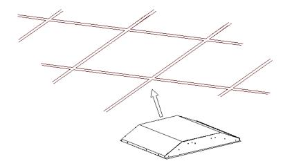
**Step 1:** Pass the troffer through the opening of the ceiling (T-grid).
